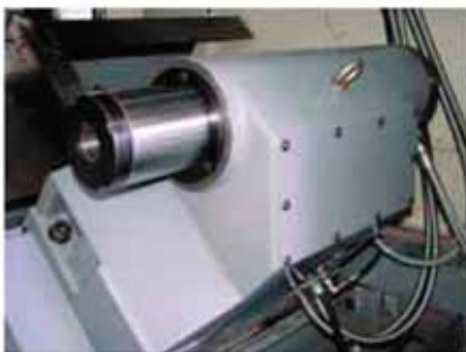
Tailstock for larger models with rotary quill.
